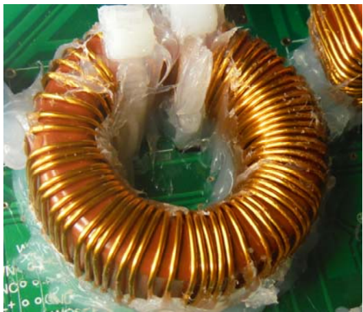
APPLY RTV I NSIDE AND ALL AROUND THE COIL
