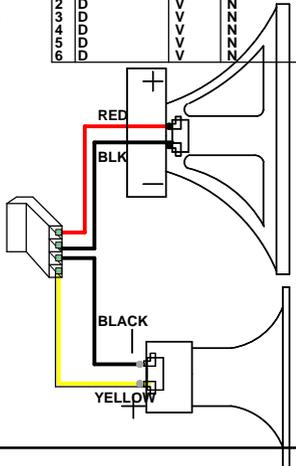
**NOTE: CONNECT YELLOW WIRE TO "HORN+" (YELLOW WIRE IS GROUND, HORN IS OUT OF PHASE)**
