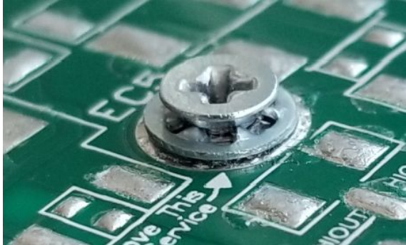
Properly inserted and seated screw and washer
