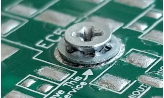
Properly fitted and seated screw and washer
