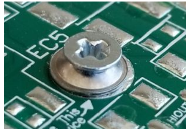
Properly fixed and seated screw and washer
