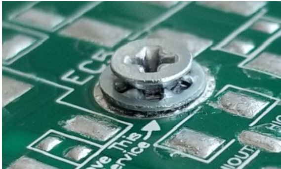
Properly fixed and seated screw and washer
