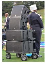
"The design of the Paraline system is a great fit for the marching audio world for its compact design, minimal power requirements, and built-in audio processing features such as level control and crossover frequencies. Even coverage of the stadium seating front to back in both level and frequency response was achieved, as expected from a line array. Only an adjustment of the level control on each box was needed to calibrate the output to each venue."
