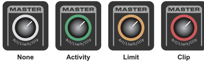
For optimal performance, the level of the system should be set such that the Act/Limit/Clip indicator is primarily green during use. An occasional indication of limiting (yellow) is acceptable, but the unit should not be operated into clipping.
